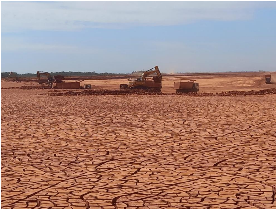
Figure 5. The new tailings management method developed by Norks Hydro at its bauxite mine in Paragominas (Brazil). The method, called Tailings Dry Backfill, allows for water removal from bauxite tailings through drainage and evaporation. This technology makes the use of dams to contain bauxite tailings unnecessary. Tailing deposition is a contentious topic in Brazil as accidents with such dams in Brazilian iron ore mines have in the recent past made many victims and caused significant environmental damage. Photo: member of Norsk Hydro’s communications team, during visit of the author, 2022.
